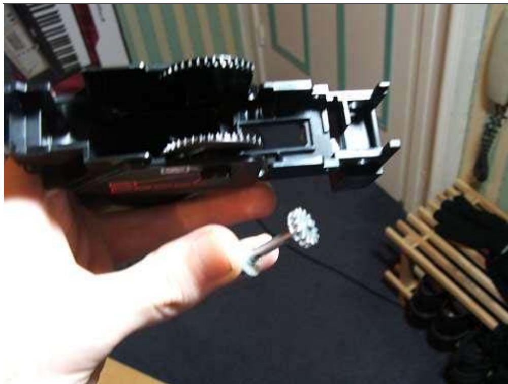
Remove the silver "pin" in the fire selector mechanism.
