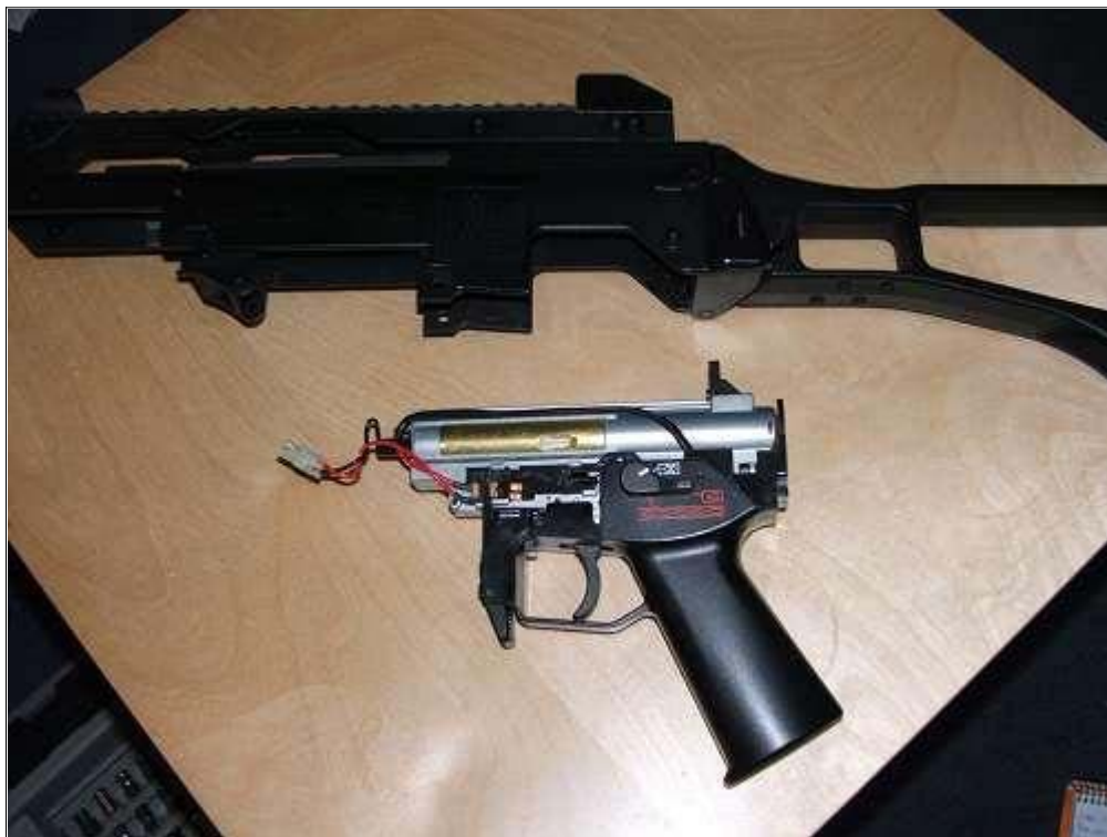
Remove the gearbox and pistol grip.
