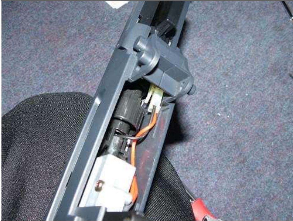
Replace the barrel assembly and electrical connection.
