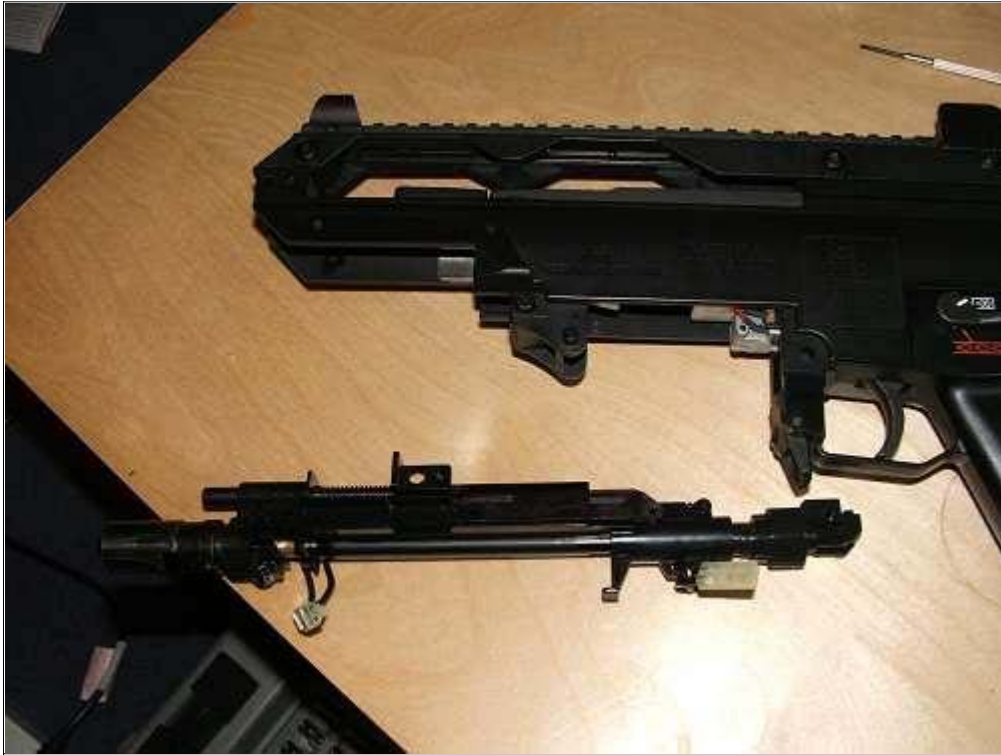
The barrel assembly after removal.
