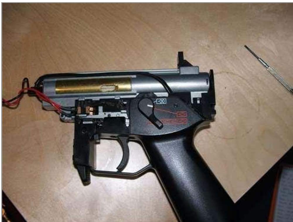
Take the gearbox out of the pistol grip.
