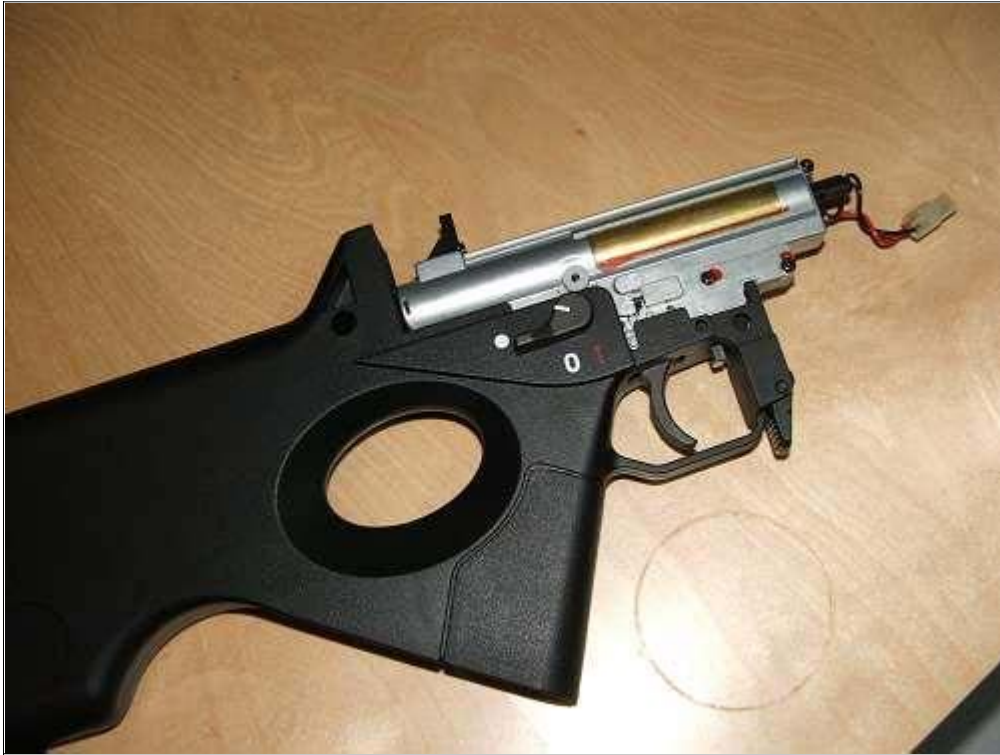
Put the gearbox back in to the stock.
