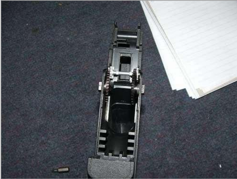
Put the two selector plates back.
