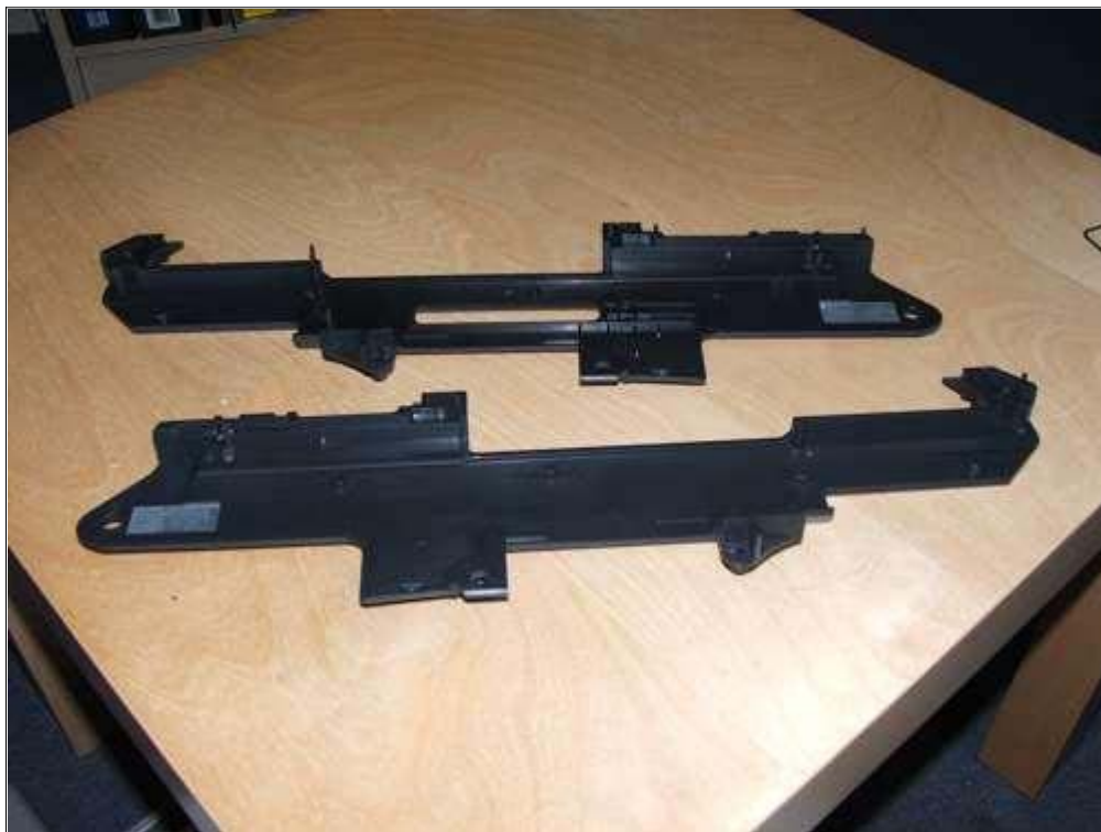
Split the SL-9 upper receiver into two halves.
