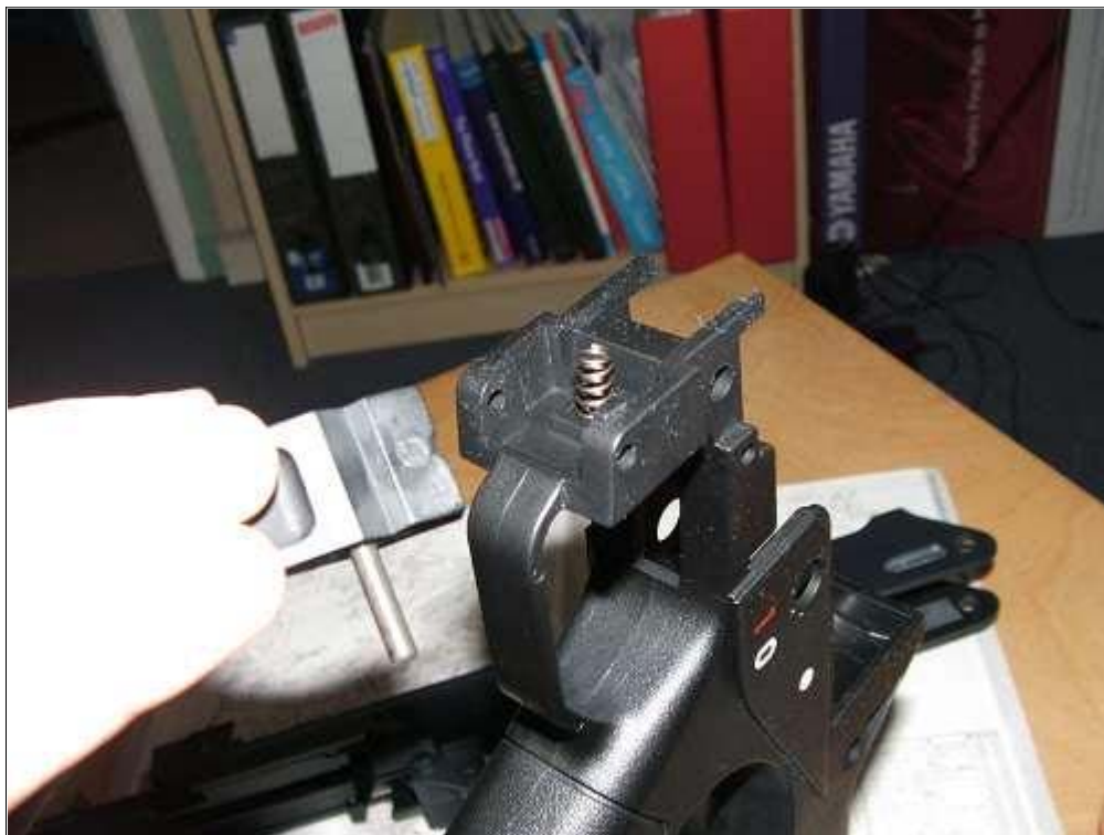
Put the magazine release lever in to the stock.
