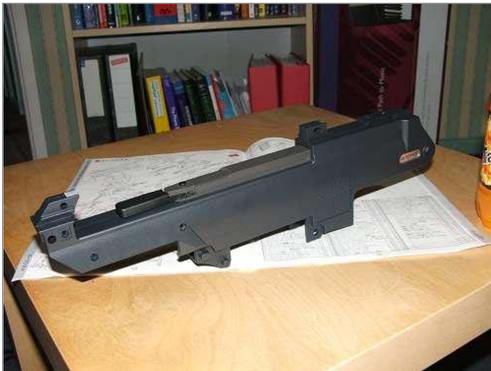
Fit the two halves of the upper receiver together.
