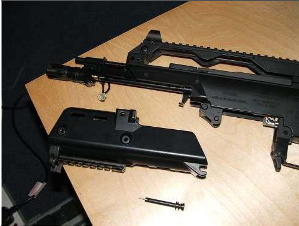
The handguard, after removal.
