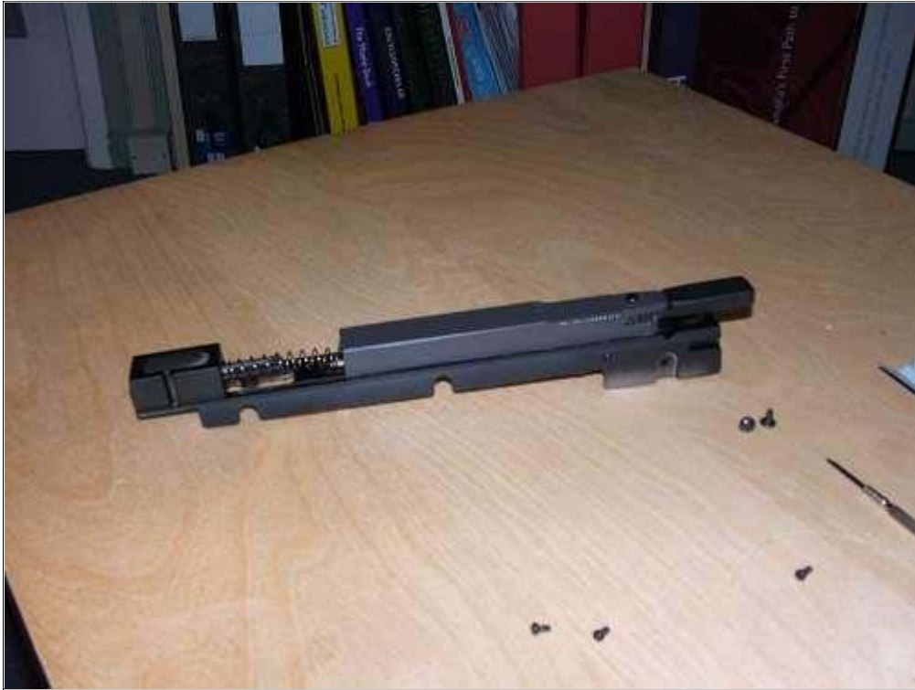
The charging handle mechanism.
