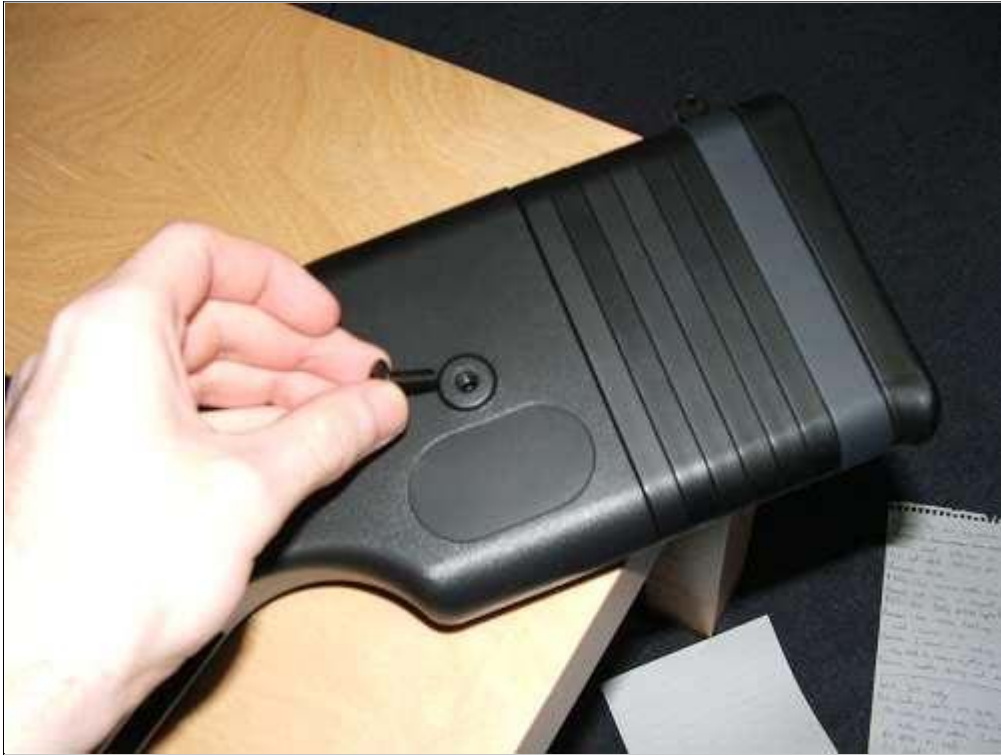
Attach the rear butt plate.
